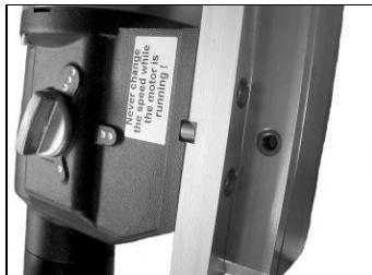
The tool is supplied with a mounting plate, a 10 mm fitting key and a 4 Allen screws M8x20. The mounting plate is put on the drill motor with the fitting key and fixed by means of the 4 screws.
