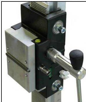
Move the machine holder upwards until it locks in the top position.
